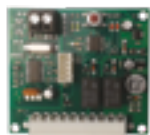
P-250RXSM2 Self-learning, two-channel, 433,92 MHz plug-in radio receiver. Accepts up to 14 rolling code transmitters
