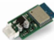
P-250T-WIFI Device for Wi-Fi connection 2,4 GHz to allow the smartphone to remotely control and program the control units via TauApp. ( P-500MASTER20T excluded )
