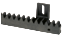
P-400CN Steel core, fibreglass reinforced, 22x22 nylon rack (Module 4, max 800 kg). Pack of 10 m
