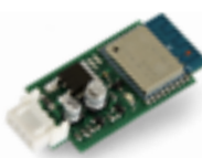
P-250T-WIFI Device for Wi-Fi connection 2,4 GHz to allow the smartphone to remotely control and program the control units via TauApp
